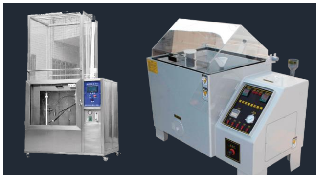
IP & Salted Water Test
